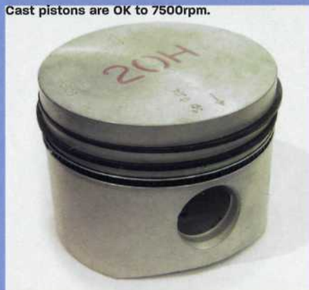
Cast pistons are OK to 7500rpm.
